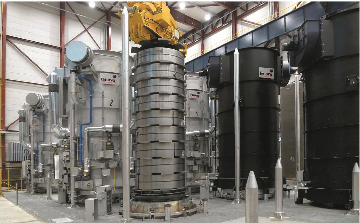
The new batch annealing plant at Bilstein comprises twelve bases; any hood fits on any free base
