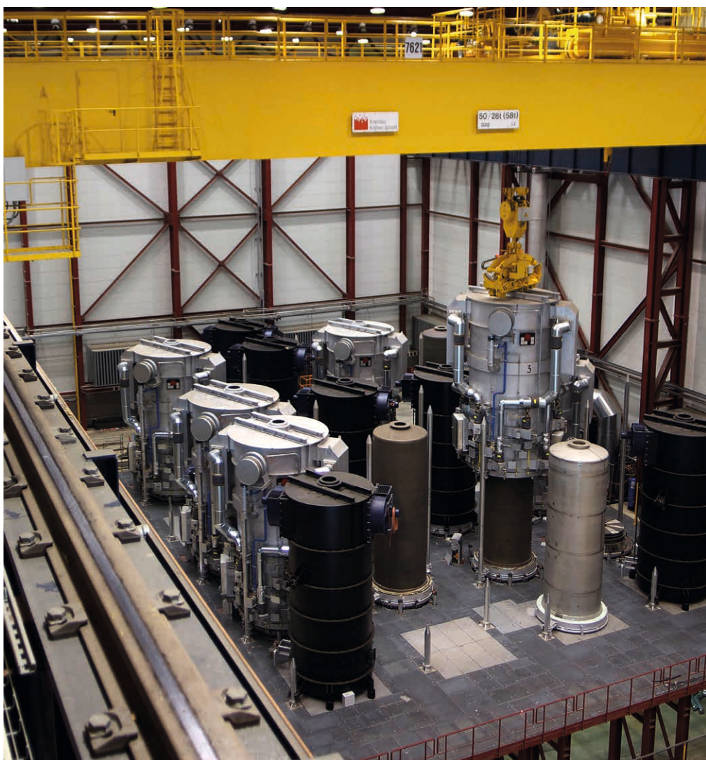
Fully automatic handling of coils, hoods and convectors (all pictures courtesy of LOI Thermprocess GmbH)
