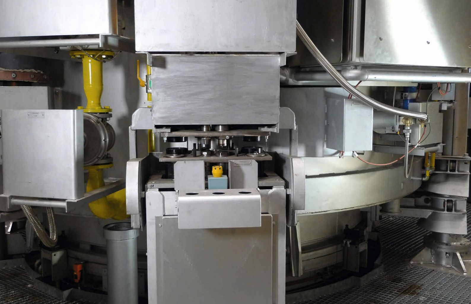
The multi-media coupling automatically establishes all connections for the gas supply (NG, H 2 , O 2 ) and the electrical signals
